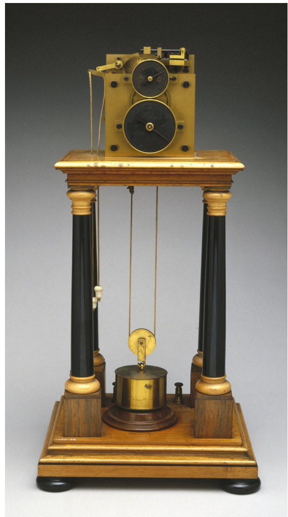
Hipp chronoscope with small galvanometer and key [Fotografía], Hipp, M., 1888, Jstor ( URL ). CC BY NC SA 4.0.
